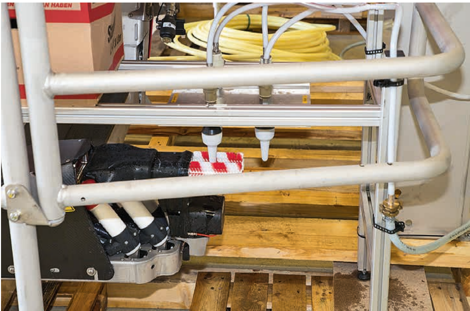
Each milking with the artificial udder started with cleaning and stimulating the teats.
